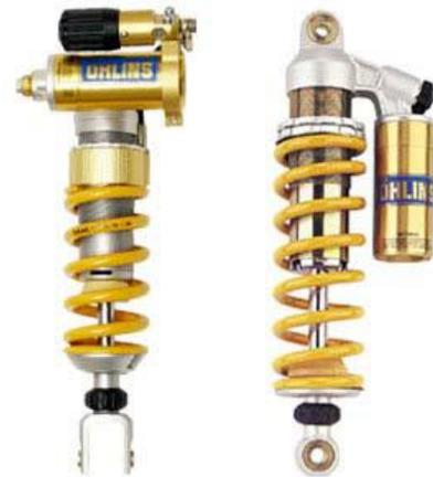
**Remote reservoir:** A shock with a reservoir unit not permanently affixed to the shock. Looks like the picture to the right ...
